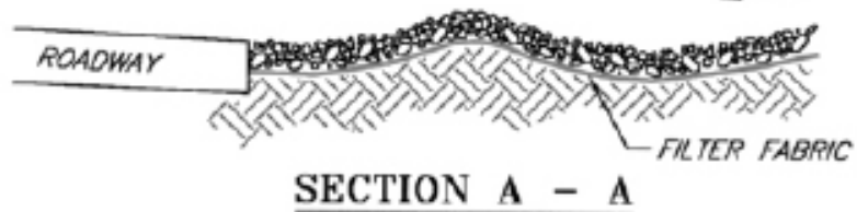
Cross Section of Water Bar Diversion
